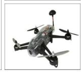
Four 2204 – 2300KV Brushless Motors, 2000mAh 3S 30C LiPo Battery, 6-Channel 2.4GHz Transmitter, 300,000 Pixel 135° FOV Video Camera 4.3" LCD FPV Video Monitor, Invensense 6050 3-Axis Gyro, Invensense 6050 3-Axis Accelerometer, 25/200mw 5.8GHz video, w/ 6 channels, Compatible with most popular FPV goggle
