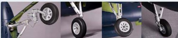
CNC-PROCESSED SHOCK-ABSORBED METAL LANDING GEAR SET
